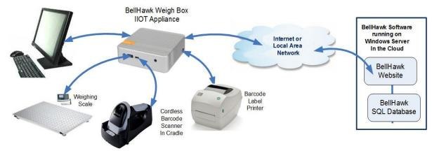
This includes using the WeighBox as a data collection station for automatically weighing materials as part of transactional data entry.
